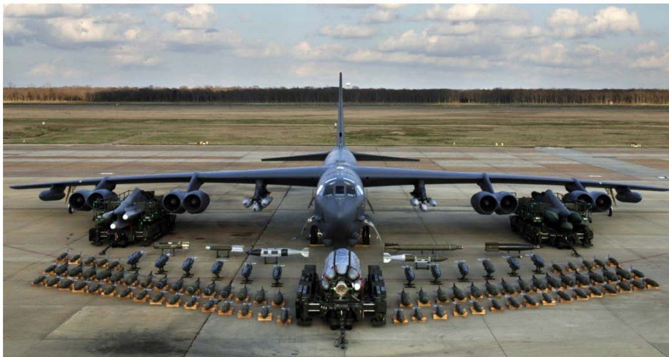
The B-52H can carry up to 70,000 pounds of conventional and nuclear weapons, including air-launched cruise missiles armed with W80 nuclear warheads and the B61 nuclear bomb. Both the B61 and the W80 were designed by Los Alamos. (Photo: U.S. Air Force)
