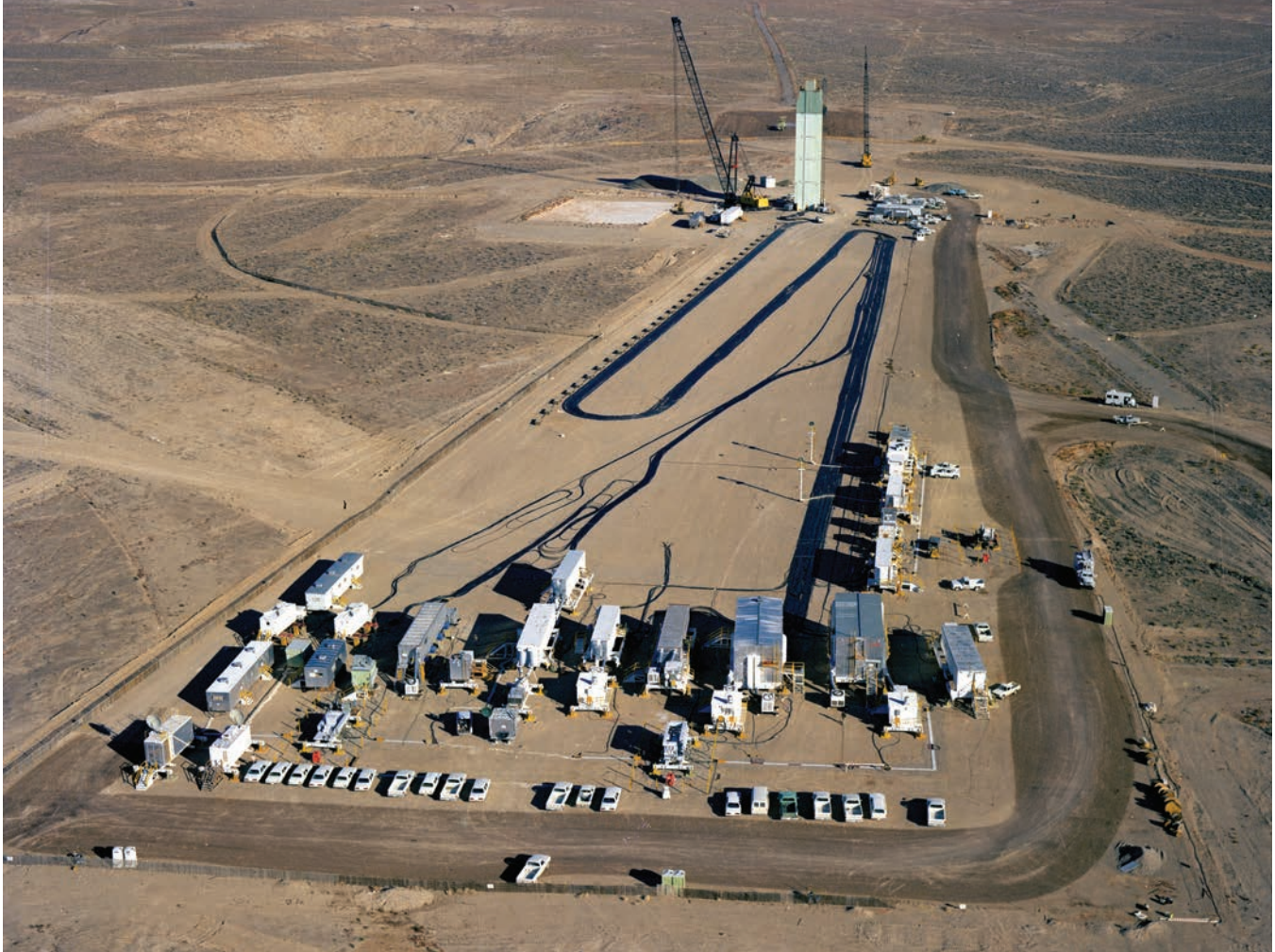
Gas-blocked cables are shown here laid out in an s-shape prior to an underground nuclear test. The cables were lowered down-hole along with a giant steel rack that contained the test device and multiple diagnostic sensors used to gather data. The cables relayed the data up to trailers (shown here in the foreground and parked at a safe distance from the detonation) containing the data recording equipment. In the background is a 10-story tower assembled around the giant rack and directly over the test hole. The tower was disassembled and removed in sections after lowering the rack but before the detonation. The tower was then reassembled over the next test hole. (Photo: DOE)
