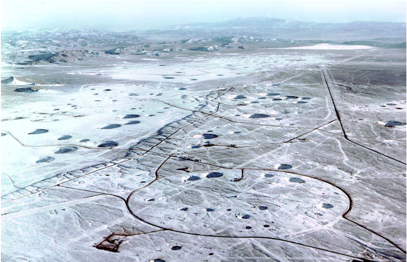
Subsidence craters—depressions on the surface that occur when the roof of the blast cavity collapses into the void left by the explosion—still mark the surface of Yucca Flat, where many underground nuclear tests were conducted at the NTS. The size of subsidence craters depends on the yield of the device, the depth of the test, and the geological characteristics of the surrounding soil. (Photo: DOE)
