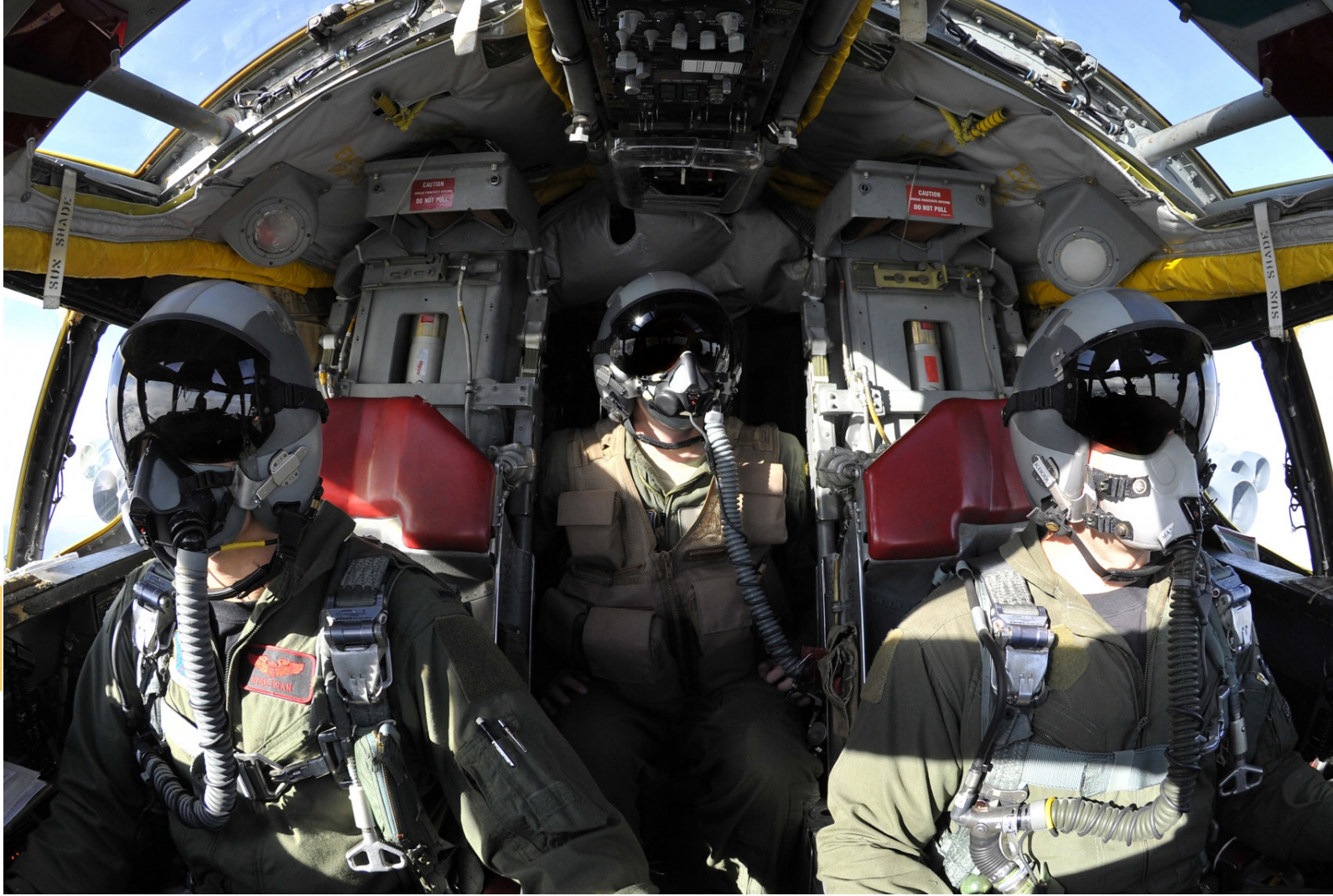
A view into the cockpit of a B-52 shows three of the plane's five crew members—the pilots and the EWO. The navigators sit downstairs. (Photo: U.S. Air Force)
