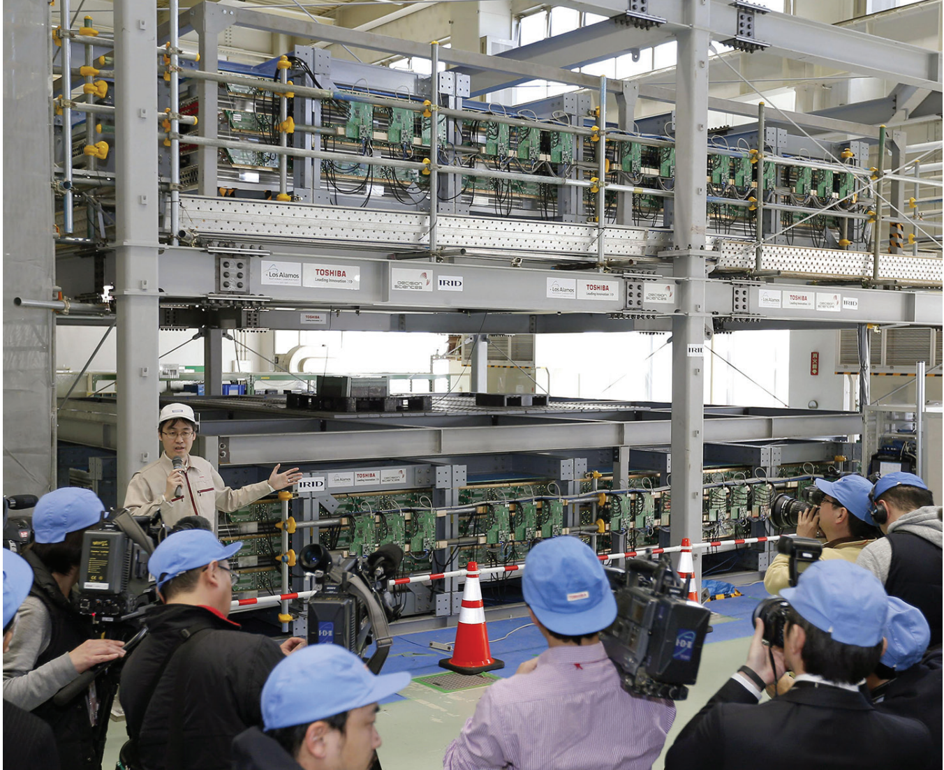
These 24-feet-by-24-feet muon detectors (one above and one behind the man addressing the crowd) will be used at the Fukushima Daiichi nuclear power plant to locate nuclear-fuel debris inside the plant's destroyed nuclear reactors. Los Alamos developed muon vision technology. (Photo: Kyodo via AP Images)
